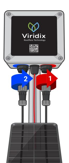
Lock the sensor wires into place with the wire clips.
