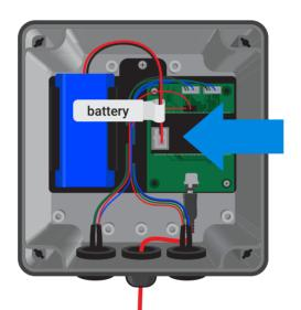
Close the Data logger by tightening the screws
