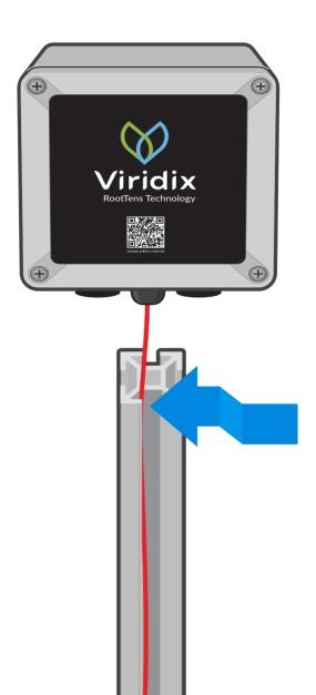
4 Slide the solar panel down the pole over the red wire.
